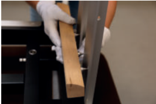
With this gauge she adjusts the distance of the side pillars to each other
